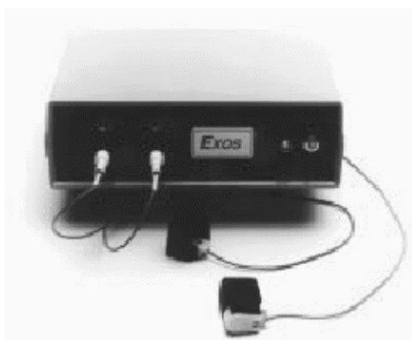
Figure 9.6: L'interface tactile TouchMaster de EXOS, copyright photo Exos
