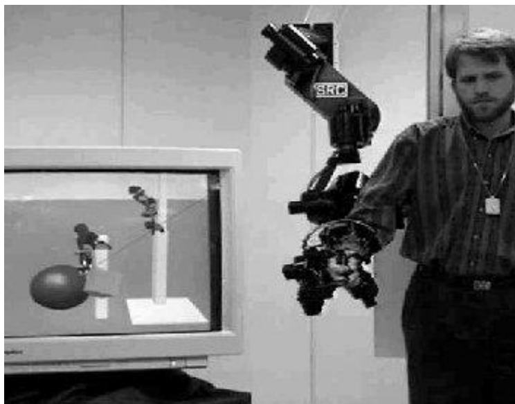
Figure 8.23 : L'exosquelette semi-portable de BDI, copyright photo Boston Dynamics
