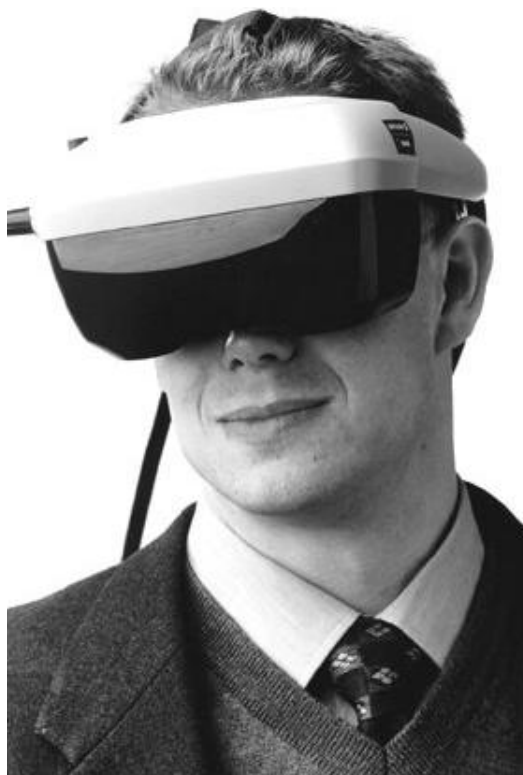
Figure 10.25 : Visiocasque AddVisor de Saab Avionics, copyright photo SimTeam
