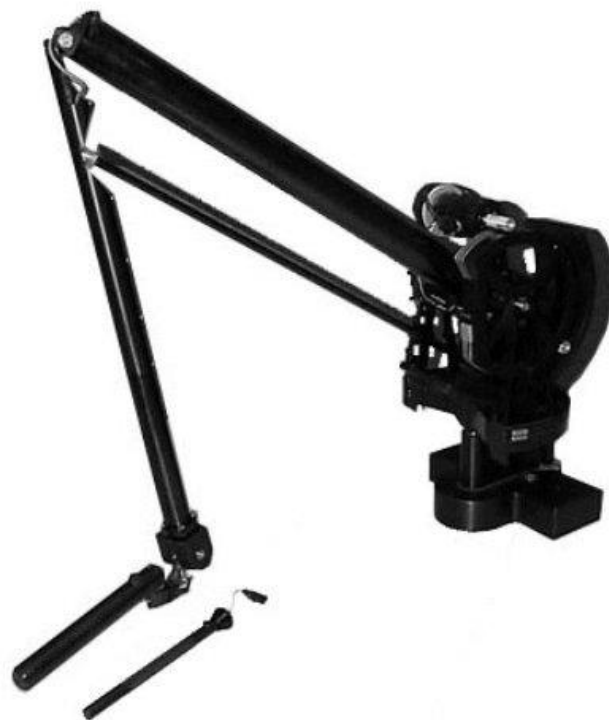
Figure 8.7: Le Phantom premium, version 3.0 de SensAble, copyright photo SimTeam
