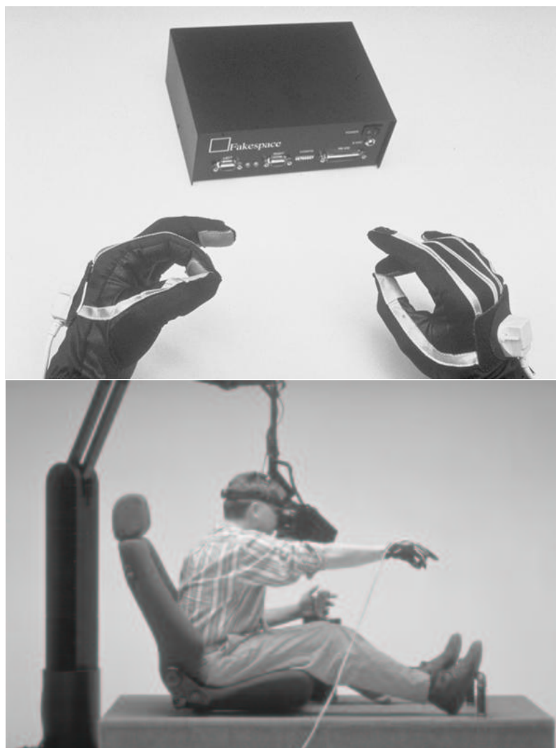
Figure 7.7 : Le gant de commandes binaires Pinch Glove de Fakespace Labs, copyright photos Fakespace Labs
