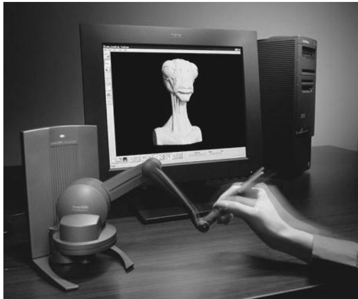
Figure 8.8: Le Phantom Desktop de SensAble, copyright photo SimTeam
