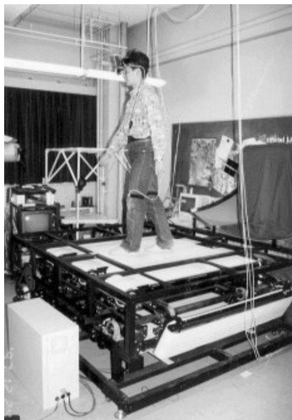
Figure 6.14: Interface de locomotion par tapis 2D Treadmill, copyright photo Professor Iwata
