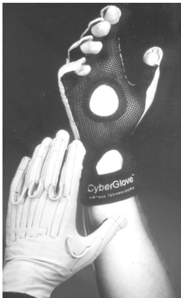
Figure 7.5: Gant CyberGlove de Virtual Technologies, copyright photo Immersion S.A.
